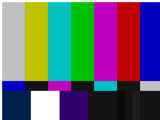
Figure 1: The SMPTE older color bars (SD) type. There is another SMPTE color bars called (HD) version with different colors.
