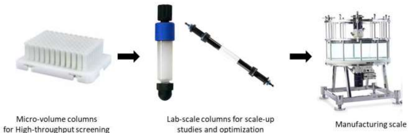
Figure 2: Scale-up strategy for chromatography
