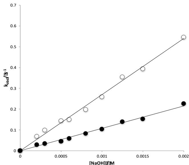
**Figure 2:** Influence of  $[NaOH]$  upon the basic hydrolysis of KCF, (O) in water ( $T=25^\circ\text{C}$ ,  $[KCF]=8.33 \times 10^{-5}\text{M}$ ) and (●) in presence of  $\beta$ -CD. ( $T=25^\circ\text{C}$ ,  $[KCF]=8.33 \times 10^{-5}\text{M}$ ,  $[\beta\text{-CD}]=6.67 \times 10^{-3}\text{M}$ ). Solid lines represent the fit of the experimental data to a line  $k_{obs}=k_2[NaOH]$ . R values are (O)  $R=0.9968$  and (●)  $R=0.9953$
