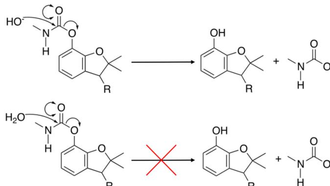
**Scheme 4:** Reaction mechanism in the basic hydrolysis of carbofuran. R: -OH, HCF and R: =O, KCF.
