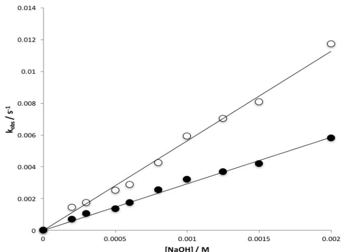
**Figure 1:** Influence of  $[NaOH]$  upon the basic hydrolysis of HCF, (O) in water ( $T=25^\circ\text{C}$ ,  $[HCF]=8.33 \times 10^{-5}\text{M}$ ) and (●) in presence of  $\beta$ -CD. ( $T=25^\circ\text{C}$ ,  $[HCF]=8.33 \times 10^{-5}\text{M}$ ,  $[\beta\text{-CD}]=6.67 \times 10^{-3}\text{M}$ ). Solid lines represent the fit of the experimental data to a line  $k_{obs}=k_2[NaOH]$ . R values are (O)  $R=0.9961$  and (●)  $R=0.9964$ .
