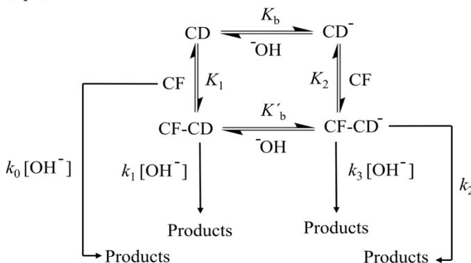
**Scheme 5:** Kinetic model for the basic hydrolysis of carbofuran-derivatives in the presence of  $\beta\text{-CD}$ .
