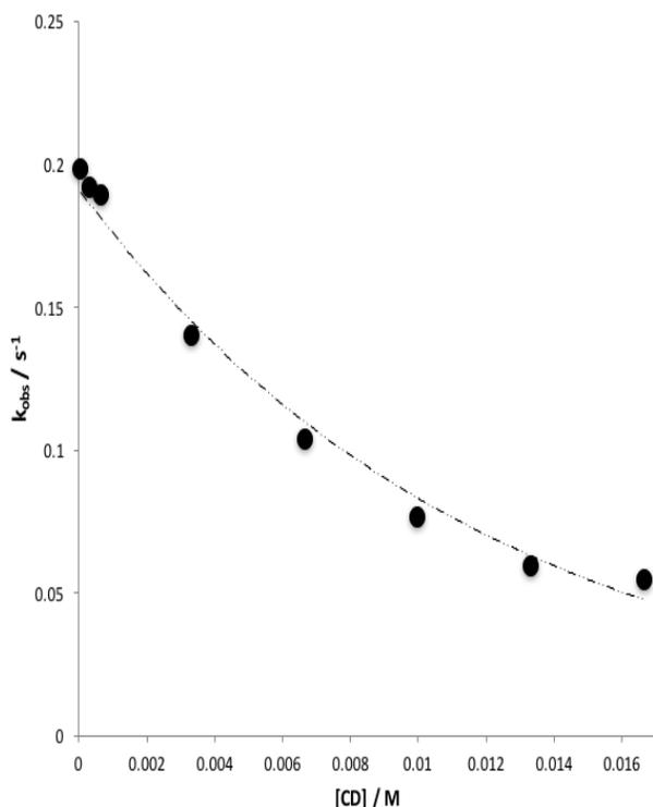
**Figure 4:** Influence of  $[\beta\text{-CD}]$  upon the basic hydrolysis of KCF ( $T=25^{\circ}\text{C}$ ,  $[\text{KCF}]=8.33\times 10^{-5}\text{M}$ ,  $[\text{NaOH}]=1.00\times 10^{-3}\text{M}$ ).
